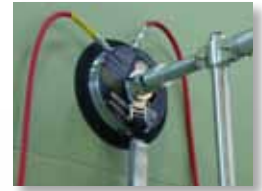
Wingrip pad secures the barrier system to the fuselage
